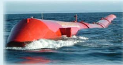
Attenuator (Pelamis) Source: Pelamis Wave Power
