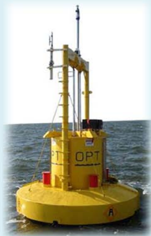
Point Absorber (PowerBuoy) Source: Ocean Power Technologies
