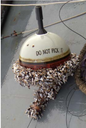
Figure 3-14. Growth of biofouling organisms on a floating spherical buoy after 521 days at sea. Source: NOAA, http://www.aoml.noaa.gov/phod/dac/gdp_drifter.html
