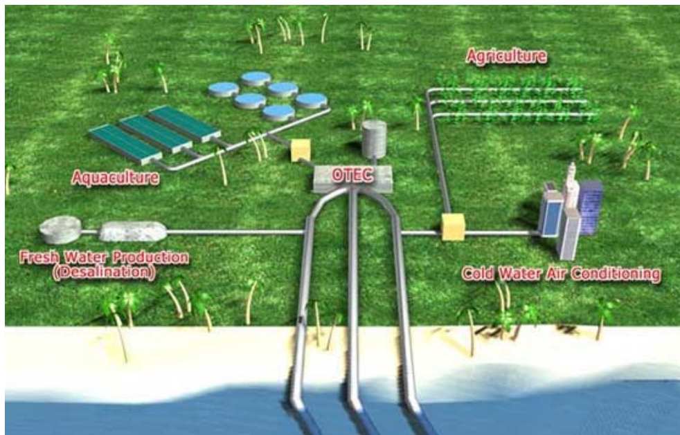
Figure 2-4. Potential co-products of an onshore OTEC electrical energy development. Source: Ocean Engineering & Energy Systems (OCEES), http://www.ocees.com/mainpages/Coproducts.html
